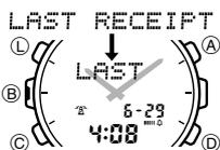
In the Timekeeping Mode, press (A) to display the date and time of the last successful receipt.
