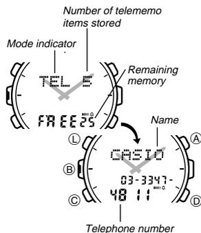
The Telememo Mode lets you store up to 30 pairs of name and telephone number data. Data is automatically sorted based on the characters of the name. You can recall data by scrolling through it on the display.
