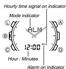
When the Daily Alarm is turned on, the alarm sounds for 20 seconds at the preset time each day. Press any button to stop the alarm after it starts to sound.
