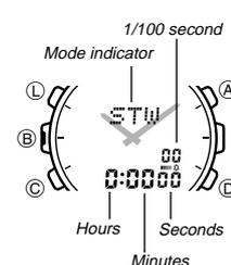
The Stopwatch Mode lets you measure elapsed time, split times, and two finishes. The range of the stopwatch is 23 hours, 59 minutes, 59.99 seconds.
