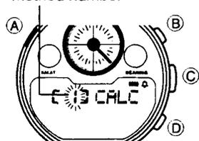
1. Press (A) while in the Timekeeping Mode. At this time, the currently set city code starts to flash on the display because it is selected.
