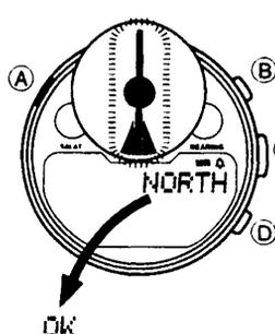
3. Place the watch on a level surface, and position it so that its 12 o'clock position points magnetic north (as measured with another compass).
