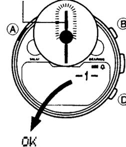
1. While in the Digital Compass Mode, press (A) to start the bidirectional calibration procedure.
