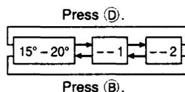
9. Use (D) and (B) to change the ISHA setting within the range shown in the illustration. Holding down either button changes the setting at high speed.
