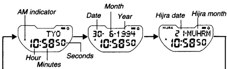
3. While the seconds digits are selected (flashing), press (D) to reset them to “00”. If you press (D) while the seconds count is in the range of 30 to 59, the seconds are reset to “00” and 1 is added to the minutes. If the seconds count is in the range of 00 to 29, the minutes count is unchanged.
