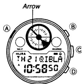
3. While in the Timekeeping Mode, press (D) to start the Qibla operation.
